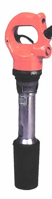
The APT Model 633 Rivet Buster measures only 20-5/8" in length, delivering more power to those tight spaces. Weighing just 28 lbs, it's perfect for limited access work or whenever a compact, lightweight and powerful tool fits the bill. This tool features an innovative cylinder design that reduces overall weight without compromising tool strength or hitting force.
