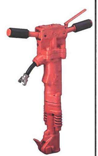
The Model 160A *Airgo*-Line® Paving Breaker is a 60 lb class tool. The ergonomically designed handle helps reduce harmful vibration to the hands and arms of the operator. This versatile tool is based on the standard Model 160, the tool being easily converted to the standard handle or ergonomic handle or vice-versa. No power is lost from the standard tool but does increase efficiency and output due to the reduction in operator fatigue.
