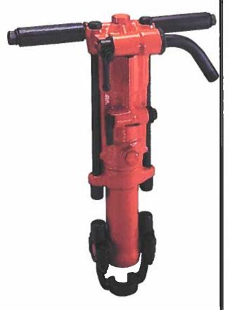
The APT Model 155 Rock Drill is a tough, 60 lb class Rock Drill. This tool can be used in general construction as well as in utility work and plant maintenance. It is designed for drilling through granite, hard faced rock, quarry drilling, and drilling secondary holes for blasting. This tool can also be used with dowel hole drilling machines. Adaptable to wet drilling applications by attaching the APT valve, wet tube and swivel assembly.
