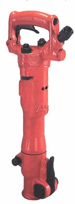
The APT Model 125 Clay Digger can be used for digging clay, shale, hard pan and frozen ground. The Model 125 is a lighter weight tool ideal for digging medium to lightly packed soil, for light demolition work as well as for tunneling around existing foundations. With its latch type retainer, lighter weight and short length, this tool is one of the best and easiest to handle Clay Diggers made today.
