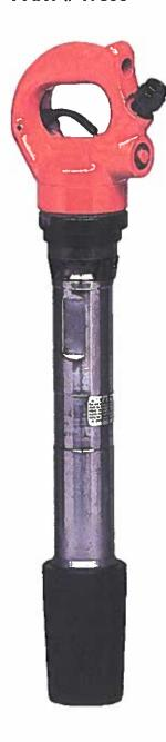
The APT Model 1133 Rivet Buster is a jumbo Rivet Buster with an 11" stroke. This model complements the "classic" 133 Rivet Buster in those applications where heavy demolition force is required. The tool is widely known as being tough and powerful, with the ability to perform heavy demolition work. Rivet Busters are also popular for cutting up underground tanks.
